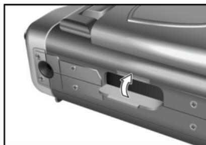
**Note:** When an SD/MMC card is not inserted, photos will be recorded in the internal 16 MB memory. However the number of photos the internal memory can store is limited to 10 ~ 20, depending on quality.
